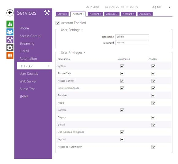
Under one of the Account tabs, enable an account that will be used to connect to the Symmetry.
