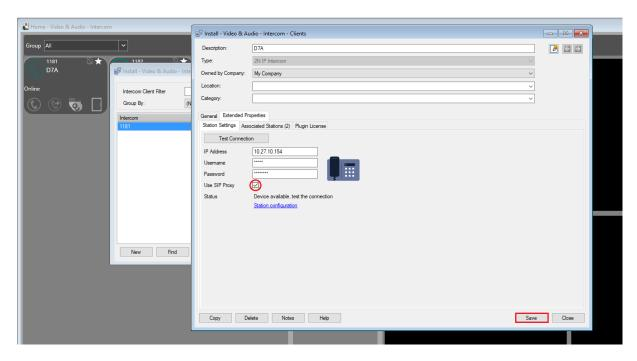
Make sure to check "Use SIP Proxy" button and don't forget to Save.
