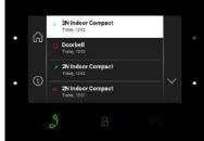
The device displays a list of all accomplished calls including date, time, status (outgoing/incoming/missed) and information on from/to which destination the call was made. The destinations that allow for some actions are white-highlighted; the other ones are gray. The side buttons and call receiving button are backlit to the maximum, the call end and lock buttons are ambiently backlit.
