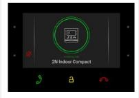
The device does not play the selected ringtone. The display shows the camera view if available, CLIP and Incoming call message. The call receiving, lock and call end buttons are backlit to the maximum. The left-hand lower button at the Mute icon and the ringing volume up/down buttons to the right are backlit to the maximum. The camera 2 (if available) switching button is backlit to the maximum. If camera 2 is unavailable, the button is not backlit and the icon is not displayed.
