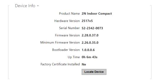
• **Factory Certificate Installed** – specify the user certificate and private key to validate the intercom right to communicate with the ACS.
