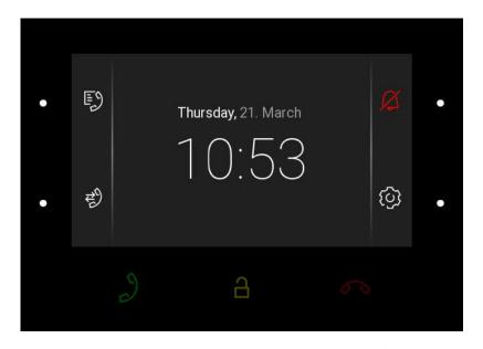
Press the right-hand upper MENU button at the icon to activate/deactivate the DND mode. When DND is active, the device is at relax and the icon is red backlit. The device does not play the selected ringtone to signal an incoming call. The display shows the camera view if available, CLIP and Incoming call message.
