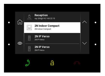
Press the left-hand upper button at the icon to display the Directory list. The menu provides a list of destinations that can be called. The destinations include their names and the device type they are equipped with. The destinations that allow for some actions (calls) are white-highlighted. The other destinations are gray.
