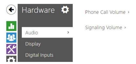
**2N** Indoor Compact is equipped with a speaker. Set the phone call and state signaling volume control in this configuration section. Master Volume controls the general device volume including call volume, signaling tone volume, and so on. Consider the noise level of the ambient environment while setting this parameter.
