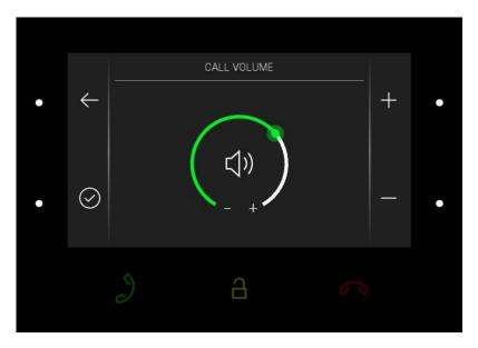
Press the right-hand upper/lower button to increase/decrease the call volume. Press the left-hand lower button to confirm the call volume level selected. The change will not be saved unless confirmed.
