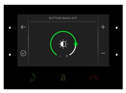
Press the right-hand upper/lower button to increase/decrease the button backlight. Press the left-hand lower button to confirm the backlight level selected. The change will not be saved unless confirmed.
