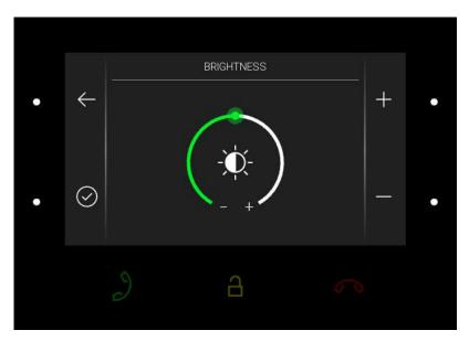
Press the right-hand upper/lower button to increase/decrease the display brightness. Press the left-hand lower button to confirm the brightness level selected. The change will not be saved unless confirmed.
