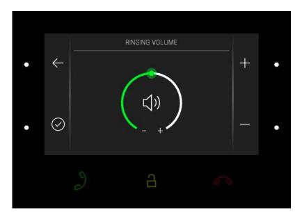
Press the right-hand upper/lower button to increase/decrease the ringing volume. Press the left-hand lower button to confirm the volume level selected. The change will not be saved unless confirmed.
