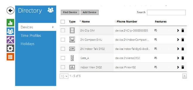
Directory is one of the crucial parts of the device configuration. It helps add new devices (2N IP intercoms and other answering units) and provides essential information on them. Up to 200 devices can be added to the directory.
