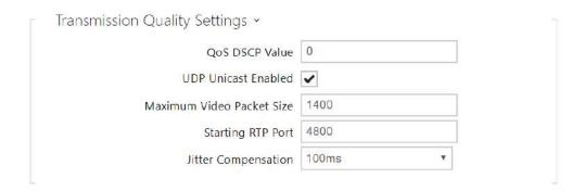
• **QoS DSCP Value** – set the audio/video RTP packet priority in the network. The set value is sent in the TOS (Type of Service) field in the IP packet header.
