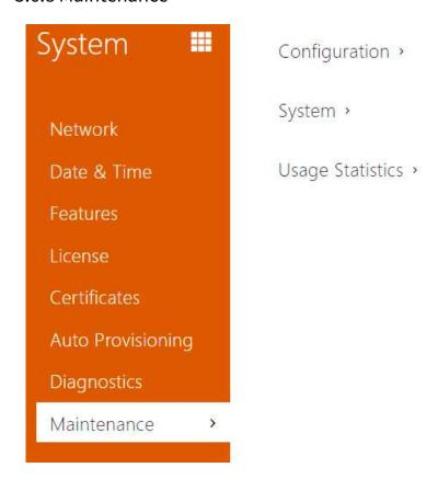
Use this menu to maintain your intercom configuration and firmware. You can back up and reset all parameters, update firmware and/or reset default settings here.
