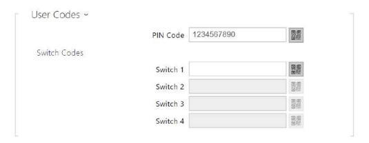
Each of the users can be assigned a unique private QR code / numerical code for switch activation. The user switch codes can be arbitrarily combined with the universal switch codes defined in the **Hardware | Switches** menu. If the codes are identical with the codes already defined in the intercom configuration, the mark will appear at the colliding codes.
