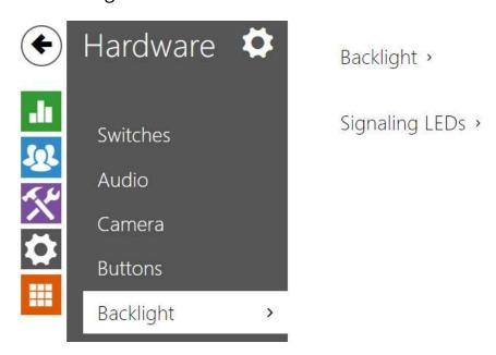
This tab helps you control the backlight level of nametags, buttons and brightness of signaling LEDs.
