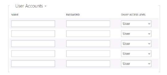
Be sure to set one user account at least and the proper access level (according to ONVIF specification and used VMS) to achieve full ONVIF functionality. Without this, the basic functionality is only available.
