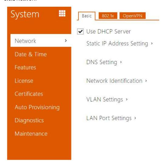
As the **2N IP intercom** is connected to the LAN, make sure that its IP address has been set correctly or obtained from the LAN DHCP server. Configure the IP address and DHCP in the **Network** subsection.
