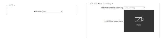
PTZ Mode – enable the PTZ (Pan-Tilt-Zoom) function to control the camera display area during the call via DTMF (GOLD license required) from your IP phone numeric keypad.
