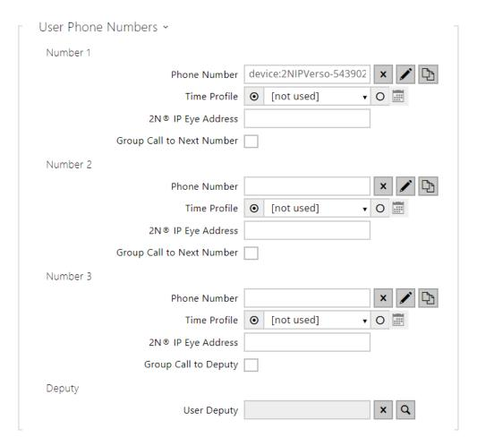
Each user in the list can be assigned up to three phone numbers. In case the user is inaccessible on one number, the following number will be dialed after a ringing timeout. Enable the **Parallel call to following number** to enable dialing multiple numbers simultaneously. The phone number validity can also be time profile-limited.
