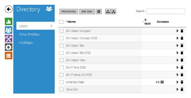
The Users list is one of the crucial parts of the intercom configuration. It contains user information relevant for such intercom functions as quick dialing, RFID card/code door unlocking, missed call e-mails and so on.
