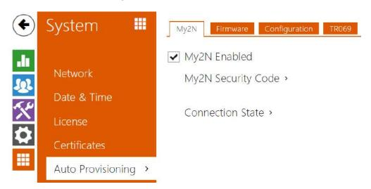
The **2N IP intercoms** help you update firmware and configuration manually, or automatically from a storage on a TFTP/HTTP server selected by you according to predefined rules.
