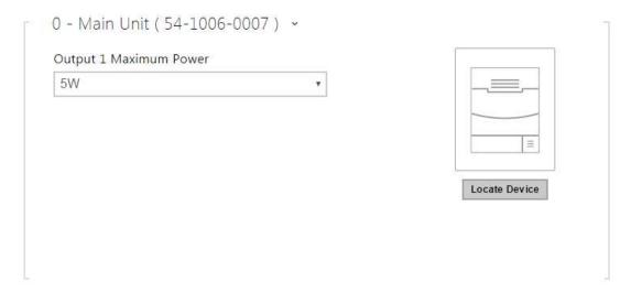
• **Locate Device** – optical and acoustic signaling of a device. Note: Optical signaling is possible only if the device is equipped with control backlight (Verso, Base, Vario, Force, Safety and Uni). If a speaker is not integrated in the device, make sure than an external speaker is connected (Audio Kit and Video Kit) to use sound signaling.
