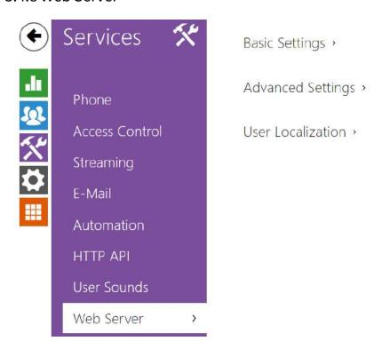
You can configure your **2N IP intercom** using a standard browser which accesses the integrated web server. Use the secured HTTPS protocol for communication between the browser and intercom. Having accessed the intercom, enter the login name and password. The default login name and password are **admin** and **2n** respectively. We recommend you to change the default password as soon as possible.
