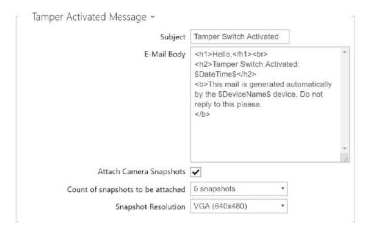
**Tamper Activated Message** – set the message to be sent to the specified e-mail address whenever the tamper switch is activated.
