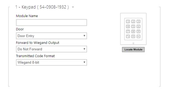
• Module Name – set the module name for logging events from the keypad.
