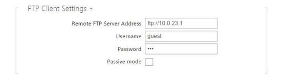
Remote FTP Server Address – set the FTP server address in the ftp://ip\_address or ftps://ip\_address format.
