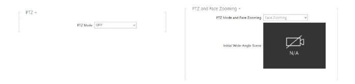
• PTZ Mode – enable the PTZ (Pan-Tilt-Zoom) function to control the camera display area during the call via DTMF (GOLD license required) from your IP phone numeric keypad.
