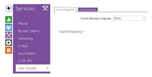
The **2N IP intercoms** provide standard signaling of operational statuses by tone sequences; refer to the Signaling of Operational Statuses subsection. If you find the standard sound signaling inconvenient, modify the sounds for the following statuses:
