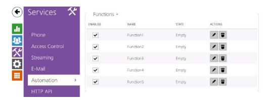
The **2N IP intercom** provides highly flexible setting options to satisfy variable user needs. There are situations in which the standard configuration settings (switch or call modes, e.g.) are insufficient and so **2N IP intercom** offers **Automation**, a special programmable interface for applications that require complex interconnections with third party systems.
