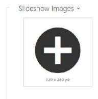
Make sure that the image resolution is 320 x 240 pixels for 2N° IP Vario. Other sizes will be adjusted to the display resolution automatically.
