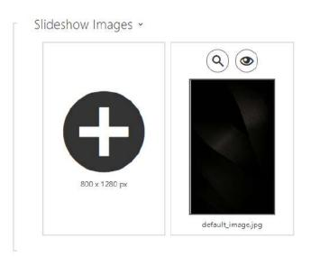
The recommended resolution is 800 x 1280 px for images and 400 x 640 px for video files in 2N<sup>®</sup> **IP Style**. The device automatically adjusts images with a different resolution value.
