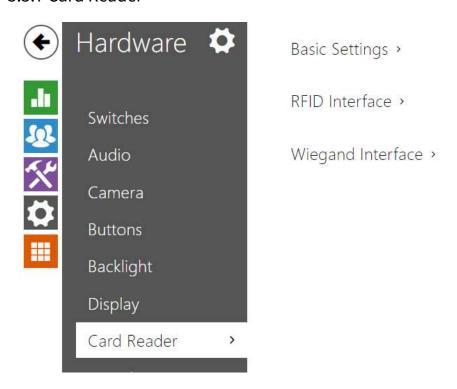
This menu is available in the **2N**<sup>®</sup> **IP Base**, **2N**<sup>®</sup> **IP Vario** and **2N**<sup>®</sup> **IP Force** models only. For **2N**<sup>®</sup> **IP Verso** only the option to limit unsuccessful access attempts is configured here. Other card reader options can be configured in the **Extenders** menu.
