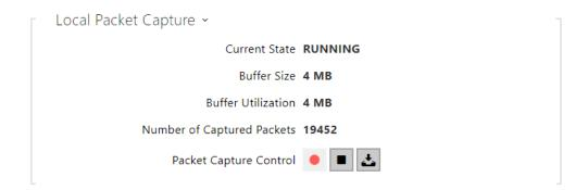
When the local capture buffer is full, the oldest packets are rewritten automatically. We recommend that you lower the video stream transmission rate below 512 kbps while capturing packets locally. Press to start, to stop and to download the packet capture file.
